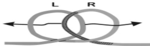
**STEP 3. Place the two loops formed over the victim's hands (or feet). Pull slack out of knot. Signal rescuers to haul**
